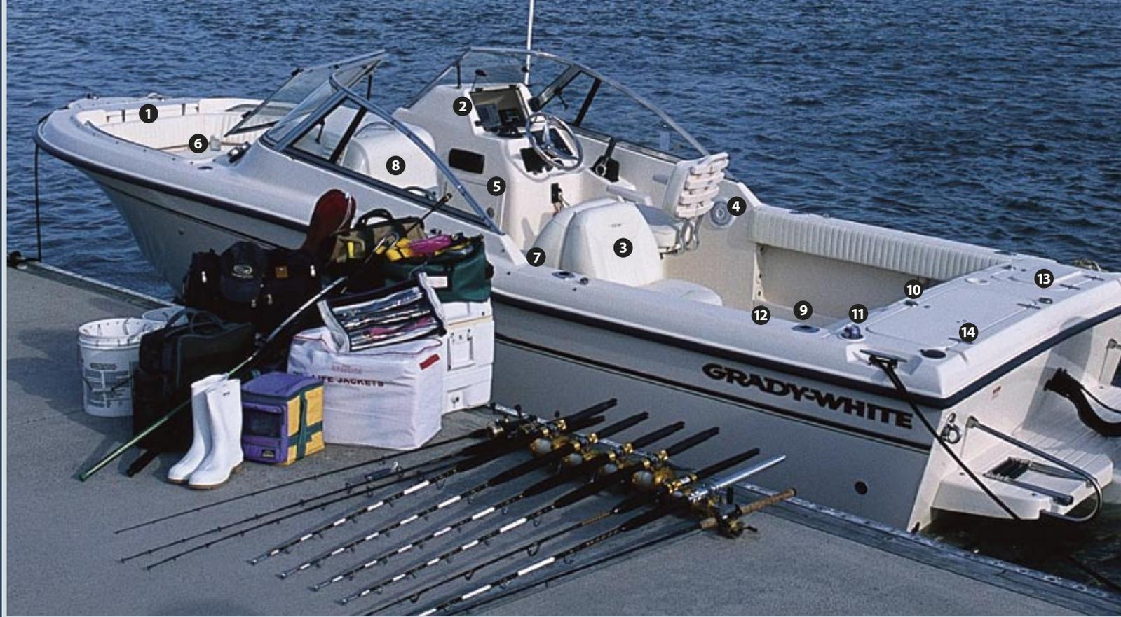
**1. The bow anchor locker** is convenient for storage and allows quick access to the anchor for safety.
