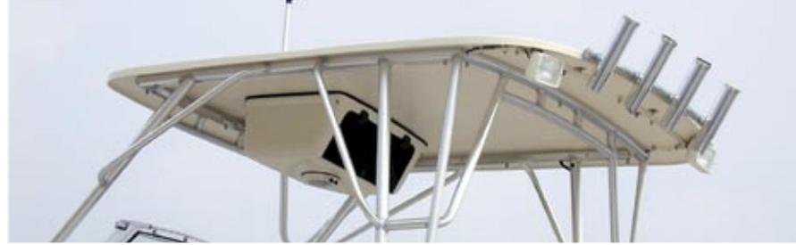
▲ Hardtop with lockable radio box, spreader lights and rod holders (208)
